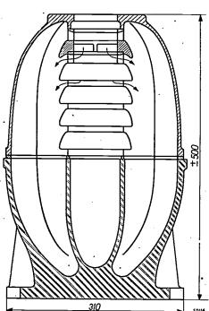
Fig. 11. Cross sections of a cooler with an inlet and outlet channel each describing 1/4 of a winding of a helix. The air distributor consists of stream-lined aluminium castings one on top of the other. The cooler housing is partly of ceramic material. The main dimensions are given in mm.
