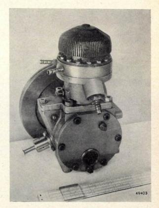
Fig. 7. Photograph of an experimental model of the single-cycle Philips air engine built according to the diagram of fig. 6. At the top is the heat exchanger of the burner, built around the heater (cf. article II). At the bottom on the left is the pump with screw for regulating the pressure. Behind the engine is the flywheel.
