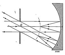
Fig. 1. A spherical hollow mirror with a diaphragm in a plane passing through the centre of curvature O. The images formed by the beams with parallel rays A and B lie on a spherical surface with  $\frac{1}{2}R$  as radius, R representing the radius of the mirror and O its centre.
