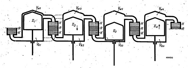
Fig. 8. Principle of the Philips multi-cylinder air engine. In each of the four cylinders is a hot space at the top,  $V_{wl}$ , and a cold space at the bottom  $V_{kl}$  to  $V_{k4}$ . The hot space of each cylinder is connected via a heater H, regenerator R and cooler K, with the cold space of the next cylinder. The pistons  $Z_1$ - $Z_4$  of the successive cylinders move with a suitably chosen phase difference (in the case shown with four cylinders this is 90°).
