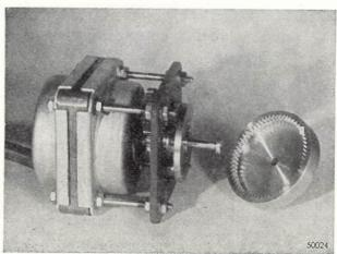
Fig. 3. A speed-reducing gearing mounted on the shaft of a small engine. Left: the apparatus ready for use. Right: the end wheel  $T_5$  has been removed for the sake of clarity. Here the transmission ratio is 500:1. In more recent constructions a modification has been made in that two or three similar toothed wheels  $T_3$  connected with each other move within the toothed rim  $T_4$ , which makes for smoother running.
