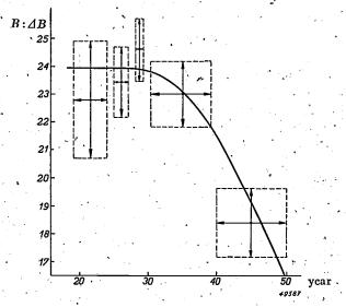
Fig. 3. Average contrast sensitivity as a function of age, measured at a level of brightness of 0.3 candle/m<sup>2</sup>, with no source of glare.
