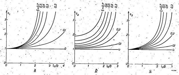
Fig. 5. The correction factors  $\varepsilon_1$ ,  $\varepsilon_2$ ,  $\varepsilon_3$  occurring in formulae (2) as functions of the ratio of slenderness  $l_0/D$  with the compression  $\xi$  as parameter.
