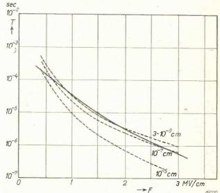
Fig. 11. Continuous line: time lag measured on the tube of fig. 10 as a function of the field strength F at the (still smooth) mercury surface.
