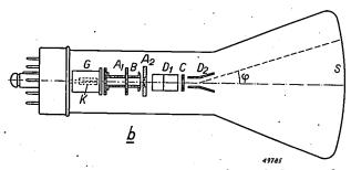
Fig. 2. Diagrammatic cross section of a cathode-ray tube, a) with pinch (type DG 7-1),
