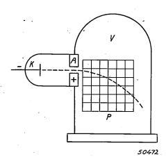
Fig. 2. Discharge vessel in which the magnetic deflection was investigated by Thomson. The rays from the cathode K pass through an opening in the anode A into the bell jar V. The curvature in a magnetic field (excited by coils of wire placed outside the vessel) is measured by causing the rays to pass along a glass plate P, upon which there is a network of lines which is photographed together with the cathode rays.
