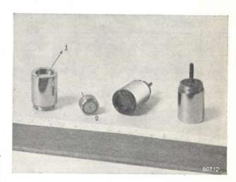
Fig. 6. Some condenser-microphones. The instrument on the left contains the diaphragm 1 stretched in the casing, and beside that is a rear electrode 2. The microphone lying on its side has a protective gauze over the diaphragm. The ruler gives an idea of the dimensions.
