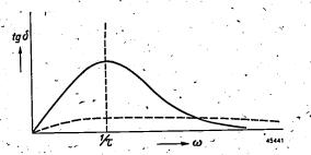
Fig. 2. The continuous line curve represents the variation of the tangent of the loss angle  $\delta$  with the angular frequency  $\omega$  according to Debije.  $\tau$  is the time of adjustment (relaxation time). The dotted line curve relates to the case where different groups of dipoles are present with different values of  $\tau$ .
