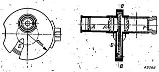
Fig. 2. Visibility meter for road lighting according to Holst and Bouma.
