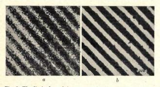
Fig. 1. The limited resolving power of a film. When a grating is pictured on the film the lines flow into each other as soon as the distance between the lines on the film becomes too small. a) Grating recorded on a film with low resolving power. b) The same grating recorded on a film with a much greater resolving power. (Taken from W. Meidinger. Die theoretischen Grundlagen der photographischen Prozesse, J. Springer, Vienna, 1937.)
