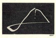
Fig. 2. Oscillogram of the secondary terminal voltage v' in a rectifier on the principle of fig. 1 with  $L_0=0$ ,  $C_0=0$ , ignition angle  $\tau_0=$  appr. 90°. Upon ignition a voltage impulse arises in the leakage inductance  $L_a$ .
