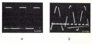
Fig. 4. a) Oscillogram of the output voltage of the new electronic switch GM 4580 (both input voltages zero); here the frequency was again about 8000 c/s. The rectangular shape is much more closely approximated than in fig. 3a.
