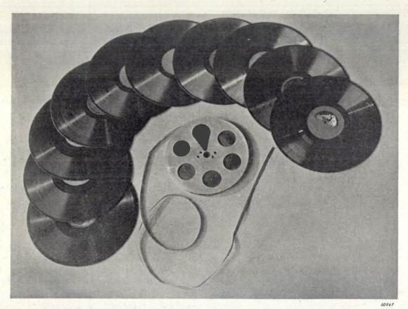
Fig. 9. An illustration of the compactness of a recording of music on cellophane film. Music that takes one hour to play can be recorded stereophonically on a film reel of the size of that shown in the illustration. For the same playing time (without stereophony!) 10 gramophone records of 25 cm diameter are required.
