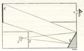
Fig. 1. Apparatus for testing night-blindness. The test person looks through the slit O in a light-proof box at a letter card placed at K. This is illuminated by one or more lamps L via the adjustable diaphragm D and the diffusely reflecting screen S. The horizontal partitions prevent any direct light from D falling upon the eye of the observer.
