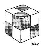
Fig. 3. The cube represents symbolically the elementary cell of the spinel lattice. The four shaded and the four non-shaded octants are occupied respectively in the same way by the metal ions, namely as in figs. 2e) and 2f) respectively.
