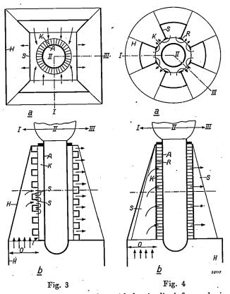
Fig. 3. Transmitting valve with longitudinal fins and air distributor. a) is the view from above on a transverse cross section at a point at half the height of the anode, b) in the left-hand half is a cross section through the plane indicated in a) by I-II, the right hand half is a cross section in the plane II-III. A, K and S have the same meanings as in fig. 2. H is the cooler housing through which the air is admitted from below via the openings 0.
