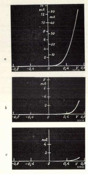
Fig. 5. Dynamic characteristics for the transmitting direction derived with the circuiting scheme of fig. 2a and, as in the case of the characteristics shown in figs. 6 and 7, recorded with an oscillograph of the type GM 3156. Amplitude of  $V_1$ : 0.68 V.
