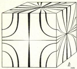
Fig. 9. Diagram of the distribution of current density in the walls of a cubic cavity resonator. The width of the "lines" is drawn proportional to the current density. The forms of oscillation a) and b) both correspond to m=n=p=1 in equation (12); the amplitudes  $(i_1, \ldots i_6)$ , however, are different in the two cases.
