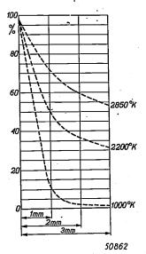
Fig. 3. Transmission of the energy emitted by three different infra-red sources (normal incandescent lamp, drying lamp, heating element of 1000 °K) through successive depths of water. Of the radiation from a drying lamp 50%, 13% and 5% is absorbed in the first, second and third millimeter respectively.
