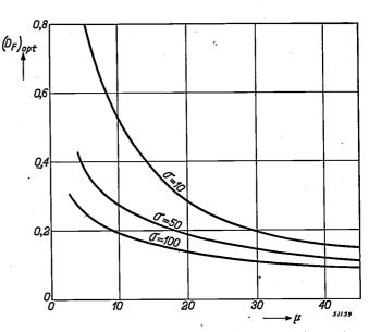
Fig. 10. The optimum thickness of the front screen (in mm) as function of the absorption coefficient  $\mu$  for three values of the attenuation coefficient  $\sigma$ . Here it is assumed that the back screen is of infinite thickness.
