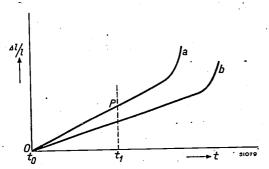
Fig. 7. Graphic representation of the expansion of two kinds of glass, a and b. The horizontal axis gives the temperature in °C ( $t_0$  is room temperature) and the vertical axis the expansion per unit of length. The expansion coefficient between  $t_1$  and  $t_0$  for glass a is found by dividing  $Pt_1$  by  $t_1 - t_0$ .
