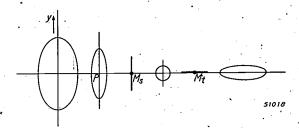
Fig. 9. Series of cross sections (H = constant) with a number of planes W (d negative, increasing in absolute value) corresponding to the terms  $Hy_0^2$  (field curvature and astigmatism).  $M_s$  is the sagittal,  $M_t$  the tangential or meridional image point. Halfway between  $M_s$  and  $M_t$  the cross section is a circle. At P (the intersection with the Petzval-surface,  $PM_s = 1/3 \ PM_t$ ) the ratio of the axes is 1:3.
