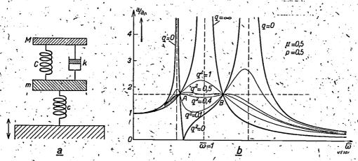
Fig. 4. Diagram (a) and frequency characteristic (b) of a vibration-free system with auxiliary mass M. The damping (k) is introduced between the main mass (m) and the auxiliary mass. The amplitude ratio is given by formula (3) on page 20. The figure here is drawn for the special case  $\mu = 0.5$  and p = 0.5, where the points of intersection A and B of all the frequency characteristics lie at the same height.
