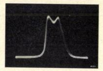
Fig. 13. Resonance curve of coupled cavity resonators recorded with the apparatus of fig. 14. The frequency is here "plotted" in the horizontal direction. The deviation in the vertical direction is a measure of the intensity of the oscillation excited in the cavity resonators.
