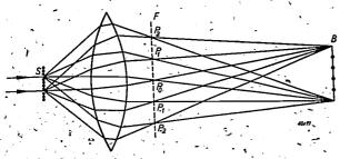
Fig. 1. Formation of the image of a grating S by an objective lens. The deflected rays converge on the focal plane F of the objective to give primary diffraction images  $P_0$ ,  $P_1$ ,  $P_{-1}$ ,  $P_2$ ,  $P_{-2}$ , etc. The image B is formed by interference of the beams coming from the primary images.
