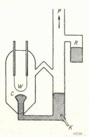
Fig. 10. Experimental tube for measuring the ignition time lag under simplified conditions. The mercury level at C is so adjusted (roughly by the addition of mercury from the reservoir R, more finely by slightly tipping the tube) as to lie at a distance of 0.25 to 0.125 mm from the tungsten strip W. The strip W is electrically heated to incandescence before each measurement in order to remove any mercury. K current lead, P pump tube.
