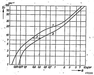
Fig. 6. The dependence of the velocity of observation  $1/\tau$  on the brightness in the case of stationary objects:
