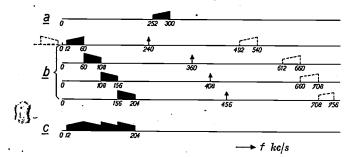
Fig. 3. Channel modulation in the 48-channel system. Twelve basic channels (a) (f = 60 - 64 kc/s) are assembled to form a basic groep (c) (252-300 kc/s) by modulating each basic channel with one of the twelve channel carriers of 192, 196.....236 kc/s (b).
