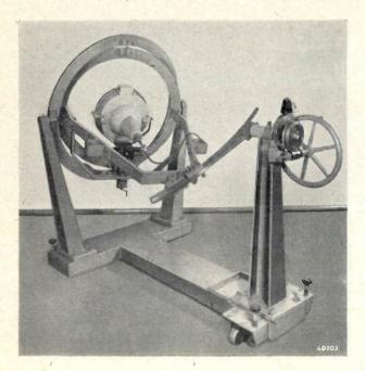
Fig. 15. The rotating apparatus when registering the light distribution of the floodlight in a different position.
