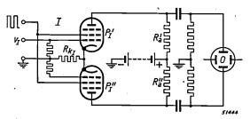
Fig. 7. Here the channel I of fig. 1 is in push-pull (pentodes  $P_{I'}$  and  $P_{I''}$ ).  $R_{kI}$  is a common cathode resistance ensuring symmetrical action.
