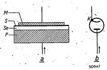
Fig. 1. a) Diagrammatic representation of a selenium rectifier. P = metal carrier plate, Se = layer of semi-conducting selenium, S = blocking layer, M = layer of good conducting metal or alloy.
