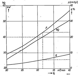
Fig. 12. Graphs relating to an anode like that of the transmitting valve TA 12/35 with a maximum temperature of 180 °C. The following are plotted as functions of the necessary amount of cold air  $V_0$  in  $m^3/\min$ : the total dissipation  $W_0$  in k, the required pressure difference p in cm water column, and the power taken up by the fan motor in percent (q) of the dissipation.
