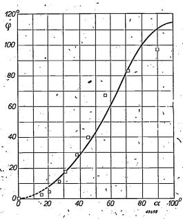
Fig. 7. Calculated elevation  $\varphi$  of an apparent source of sound straight ahead, as function of the distance to the two loudspeakers (angle a). For very great distances (small angle a) the calculation is rather unreliable; the curve for this range is drawn in a broken line. The squares are the mean values of the series of measurements given in fig. 3.
