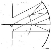
Fig. 10. A diaphragm the centre of which coincides with the centre of the mirror M brings about a practically sharp image on a sphere with radius |f|=R/2. Depending on the diameter of the diaphragm, however, spherical aberration occurs. The point sources  $P_0$  and P are to be imagined as the infinitely distant points of the main and secondary axes respectively.
