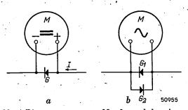
Fig. 13. a) Direct current meter M safeguarded against overload by the rectifier G connected in parallel.
