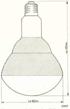
Fig. 6. Dimensions and shape of a Philips drying lamp.
