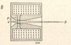
Fig. 5. Drawing of a cross section of a magnetic lens enclosed in an iron jacket, a without, and b with pole shoes. In these figures F are the lines of force, S is the slit, P the pole shoes. At V is the object and at B the image. In case a the focal distance may amount to several centimetres and in b to several millimeters. In connection with the vacuum which is maintained inside the microscope, the slit in the iron jacket is closed by a copper ring.
