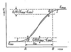
Fig. 8. The S-shaped curve I represents the energy distribution in an edge image with a screen blurring of the same magnitude as the kinetic blurring  $u_m$  to which the energy distribution according to the straight line II corresponds. The straight line passes through the points a and b for which  $E-E_{\min}=0.16$  ( $E_{\max}-E_{\min}$ ) and 0.84 ( $E_{\max}-E_{\min}$ ) respectively. The distance AB, which in this case is 0.92 mm, is a measure of the screen blurring.
