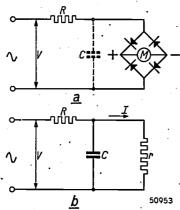
Fig. 11. a) Circuit for measuring alternating voltages with the aid of a moving-coil meter M, a Graetz circuit of four cells and a series resistor R. By means of the broken line capacity C allowance can be made for the capacity of the cell.
