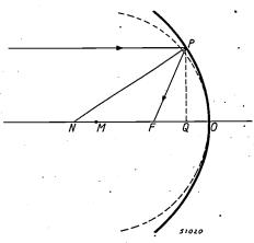
Fig. 11. The passage of rays with a parabolic mirror. A ray through P parallel to the axis, after reflection, strikes the axis at F,  $MF = FO = \frac{1}{2} |R|$ . Here R is the radius of curvature at O (broken line). NP is the normal drawn from P on the parabola; NQ = MO = |R|.
