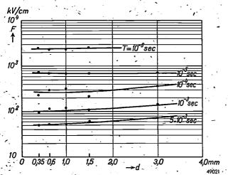
Fig. 12. The field strength F necessary to obtain a given time lag T is found to depend only little on the thickness of wall d of the diclectric igniter.
