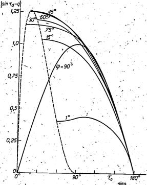
Fig. 6. The factor  $|\sin \tau_d - q|$  by which the voltage impulses upon extinction are proportional, as function of the ignition angle  $\tau_0$ , with  $\varphi$  as parameter. The curves end to the left on the dotted limit line, for which the equation (13) applies; this has a maximum of 1.26 at  $\tau_0 = 18^\circ$ . The extinction impulses are large with many combinations of  $\varphi$  and  $\tau_0$  where  $\varphi \approx 15^\circ$ -90°,  $\tau_0 \approx 15^\circ$ -120°.
