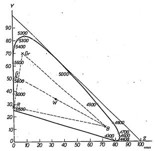
Fig. 1. In this colour triangle the colour point is plotted of the emission of a blue (B) and a yellow (G) luminescent substance. When two colours are mixed a new colour is formed, which is represented by a point on the line connecting the colour points of those two colours. White (W) lies on the line connecting blue and yellow. Further it is clear that white can also be obtained from the addition of a red, a green and a blue colour (R, Gr and B).
