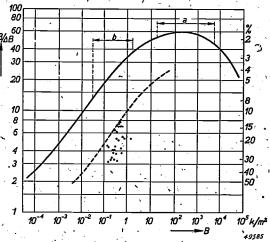
Fig. 1. Dependence of the contrast sensitivity  $B/\Delta B$  on the level of brightness B. In road lighting (brightness range b) this is less than in daylight (range a).
