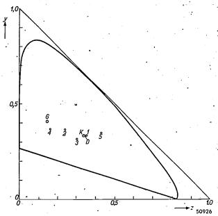
Fig. 5. The colour points of the eight sources of light used here. G = incandescent lamp, K = artificial daylight, D = natural daylight, I-5 experimental low-pressure mercury lamps coated with different fluorescent substances.
