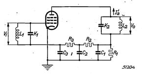
Fig. 5. The same circuit of fig. 4 with the addition of two circuits  $L_1$ - $K_1$  and  $L_2$ - $K_3$  tuned to the signal frequency.
