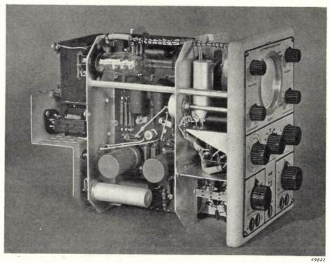
Fig. 11. An internal view of the oscillograph GM 3159. The compartment on the left contains the supply unit, the one in the middle the two amplifiers. The empty space on the left can be reached through a trap in the back of the casing and can be used for storing away the flexes.
