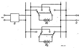
Fig. 1. Two-battery system. While the battery  $B_2$  is feeding the plant connected at O the battery  $B_1$  is being charged by the rectifier G. When battery  $B_2$  becomes exhausted two switches are thrown over and the functioning of the batteries is interchanged until  $B_1$  is exhausted, and so on.
