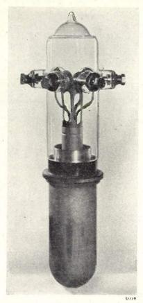
Fig. 2. A transmitting valve. A number of metal caps are fused air-tight onto the glass. At the bottom a so-called "can" is affixed to the glass by means of a chromium iron intermediate piece.
