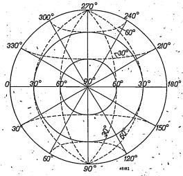
Fig. 11. The azimuthal projection of a spherical grid according to Lambert. The full lines represent some meridians and circles of latitude of a system of coordinates whose polar axis is perpendicular to the drawing plane. The dotted lines are some meridians and circles of latitude of the system of coordinates corresponding to the rotating apparatus of fig.
