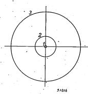
Fig. 7. Intersection figures on the plane V corresponding to the terms with  $H^3$  (spherical aberration) for values of H which are as 1:2:3.
