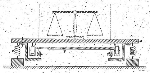
Fig. 2. Model of the practical construction of a vibration-free mounting with auxiliary mass. The plate p supported by the helical springs c and carrying the instrument represents the main mass, the plate P connected below with the helical springs C is the auxiliary mass. Between these two plates the damping k has been provided.
