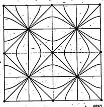
Fig. 4. The occurrence of a higher characteristic oscillation of a square plane cavity resonator. This may be conceived of as the result of placing four smaller square resonators side by side, each of which executes the fundamental oscillation. The points indicate the spots where the current density becomes equal to zero.
