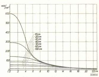
Fig. 8. Graphic representation of the distribution of the radiation intensities (in mW/cm²) in planes perpendicular to the lamp axis at different distances away from the lamp varying from 10 to 100 cm. The horizontal axis gives the distance between the point in question and the lamp axis.
