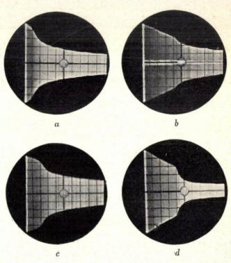
Fig. 2. Photographs of cooling curves obtained with different oils. The max. vertical deflection corresponds to 800 °C and the horizontal to 23 secs.
