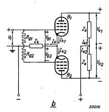
Fig. 3. Two methods of obtaining from a push-pull amplifier a symmetric output voltage
