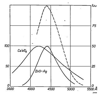
Fig. 12. The full lines represent the spectral distributions of the light emitted by a CaWO<sub>4</sub> screen and a ZnS-Ag screen. The intensity is given along the vertical axis on the left on an arbitrary scale. The dotted line represents the relative spectral sensitivity of a non-sensitized photographic film, derived from measurements with Agfa Spectral and Ilford Spec. Rapid films; the corresponding scale is given on the right..
