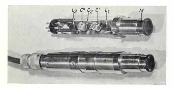
Fig. 8. Top: Opened condenser-microphone showing the component parts built in. M is the microphone proper;  $L_1$ ,  $L_2$  and  $C_2$  have the same meaning as in fig. 6; the small adjusting condensers (trimmers) C' and C'' are connected in parallel to the microphone and to  $C_2$  respectively. Bottom: The microphone encased and connected to a cable,
