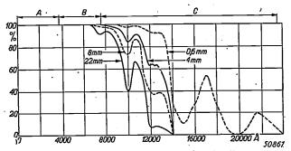
Fig. 2. The transmission of infra-red rays of different wavelenths through layers of water of different thickness. It appears that the layers of 22, 8 and 4 mm thickness absorb all energy of wavelengths above 14 000 Å.
