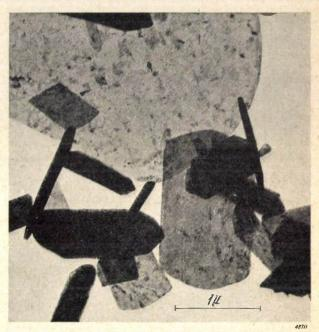
Fig. 13. Molybdenum oxide magnified 30 000 times electronbptically with an accelerating voltage of 82 kV.
