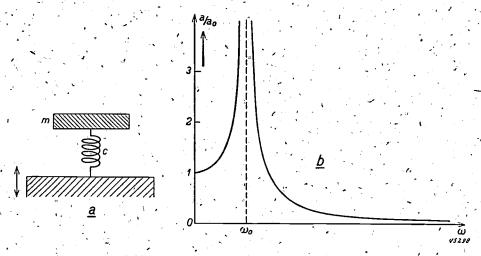
Fig. 1. Diagram (a) and frequency characteristic (b) of an undamped, vibration-free system. At frequencies  $\omega$  which lie far enough above the resonant frequency  $\omega_0$  the amplitudes of the forced vibrations of the mass m caused by the vibration motion of the foundation are very much reduced. The amplitude ratio is:  $\frac{a}{a_0} = \left| \frac{c}{c - m\omega^2} \right|$ .
