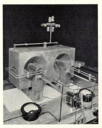
Fig. 10. An induction-tube oscillator of high power. The two induction tubes are mounted in the cavity resonator at the point of voltage maxima. In this way use is made of the fact that at higher forms of oscillation a cavity resonator has more than one voltage maximum.
