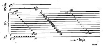
Fig. 7. Modulation diagram of the 12-channel system introduced in the Netherlands in 1935. Double modulation with a basic channel at 60-64 ke/s and final allocation of the channels in the 8-56 kc/s frequency band.
