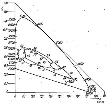
Fig. 2. . Positions of the colour points of the ne-cards of Ostwald in the I.C.I. mixture diagram. The broken-line polygon connects up the colour points obtained under incandescent lamplight, whilst the fully-drawn polygon appertains to artificial daylight. G and K are the colour points of the two kinds of light themselves.
