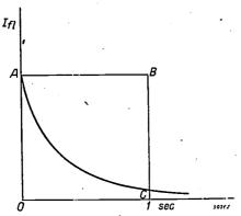
Fig. 3. Reduction in the intensity of fluorescence in a plan-position-indicator after the cathode-ray beam has passed. On the  $\alpha$ -axis is the time and on the  $\beta$ -axis the intensity of the fluorescence. The broken line ABC represents the ideal intensity change and the curve the approximation hitherto reached.
