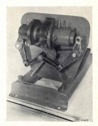
Fig. 2. Experimental model of an air engine constructed according to the principles of fig. 1. The position of the parts is the same as in fig. 1.
