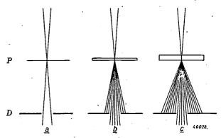
Fig. 1. The scattering of the electrons by objects of different thickness. In a, b and c rays are drawn which pass respectively through a very thin, a medium and a thick specimen P. D represents the objective aperture which captures part of the electrons in each case. In thick parts of the specimen the scattering is so great that only a small number of the rays reach the image. As a result the part of the image corresponding to a thick part of the specimen will be much "darker" than the rest.
