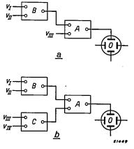
Fig. 13. Block diagram for the simultaneous recording of (a) three or (b) four oscillograms. A, B, C = electronic switches, O = oscillograph tube,  $v_I \dots v_{IV} =$  input voltages.
