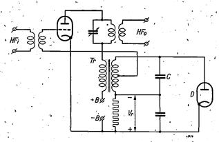
Fig. 6. H.f. amplifier (input  $HF_i$ , output  $HF_o$ ) analogous to that of fig. 5 but with the l.f. auxiliary signal generated in the amplifier itself (oscillating circuit with feedback, consisting of transformer Tr and capacitor C). The l.f. voltage is rectified by a diode D and forms directly the control voltage  $V_2$ , used for compensating deviations in slope. +B and -B are poles of the anode voltage source.
