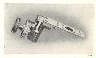
Fig. 6. Berek's compensator. A small plate of calcareous spar is placed obliquely in the pencil of rays by means of a micrometer screw. The magnitude of the double refraction thus set up is determined from the reading of the scale on the screw.
