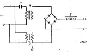
Fig. 4. Arrangement of a normal rectifier with transformer T, four selenium valves V with Graetz circuit, and smoothing choke S.
