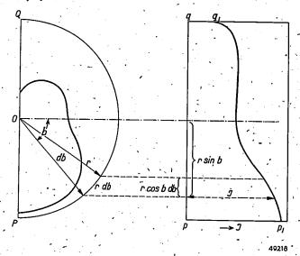
Fig. 2. The calculation of the total luminous flux of a rotation-symmetrical light source with the aid of the Rousseau diagram from the polar graph of the candle power distribution measured in a meridian plane. Here r is the radius of the sphere imagined around the light source, b the latitude in the system of coordinates and I the measured candle power. The area of the figure  $pp_1q_1q$  is proportional to the total luminous flux  $\Phi$ .
