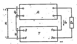
Fig. 1. The output a.c. current  $I_a$  from an amplifier A is conducted to the input terminals 1-3 of a feedback system T. At the output terminals 2-4 there consequently arises a voltage  $V_t$  which together with the input signal  $V_t$  forms the voltage  $V_g$  supplied to A. The + and - signs at the terminals indicate in what direction the a.c. voltages  $V_t$ ,  $V_t$  and  $V_g$  are positive.  $Z_o$  is an external impedance.
