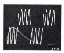
Fig. 11. Oscillograms recorded with a low commutating frequency  $(f_c < f_i)$ . The frequency of the time-base voltage has been chosen low enough for the image to cover two cycles of the commutating frequency.
