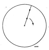
Fig. 2. A cathode-ray beam causes a narrow linear part of the screen of the plan-position-indicator to light up. This ray travels round the screen in about 1 second while the cathoderay beam moves up and down that ray at a high velocity.
