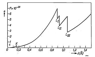
Fig. 3. Graph representing the absorption a as function of the wavelength  $\lambda$  for the element Pb. The single K-absorption edge and the three-fold L-absorption edge occur when the quantum of X-rays is large enough to release an electron from the K and the L shells respectively.
