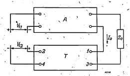
Fig. 3. When for a certain frequency the transfer impedance  $Z = V_{tz}/I_a$  of the feedback system T assumes the value -1/S (eq. (8)) then the voltage supplied by T is just identical with the voltage required at the input of the amplifier A to produce  $V_{tz}$ . When the output of T is connected to the input of A the amplifier begins to oscillate in that frequency.
