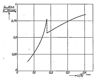
Fig. 11. The ratio of the quantities  $(k_{re}G)$  ZnS and  $(k_{re}G)$  CaWO<sub>4</sub> (for  $\sigma = 50$ ) as function of the wavelength  $\lambda$ . Here  $k_{re}$  represents the efficiency of the transition from X-rays into electron energy, whilst G is the function illustrated in fig. 8.
