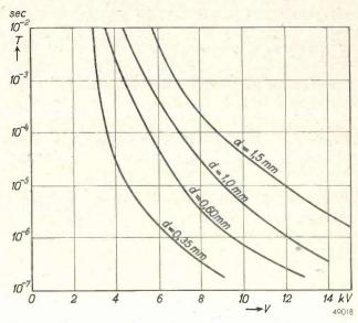
Fig. 8. The oscillographically determined real time lag T as a function of the voltage V applied to the starter; d is the thickness of the wall of the starter.
