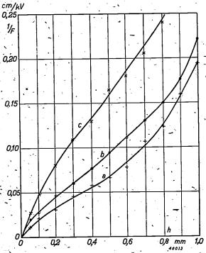
Fig. 4. Field strength F at the mercury surface at a voltage of 1 kV on the igniter. 1/F (F in kV/cm) is plotted as a function of the height h above the boundary between the mercury and the starter wall. Curves a, b and c are for walls with  $\varepsilon = 4.4$  respectively 0.35, 1.0 and 3.0 mm thick. They are derived from measurements described in the article cited in footnote  $^{5}$ ).
