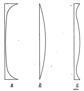
Fig. 3. a) A correction plate for a Schmidt optical system.
