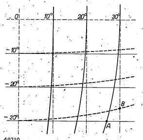
Fig. 9. The middle part of the diagram illustrated in fig. 8 on a magnified scale. The bearing indicated by  $30^{\circ}$  north and  $30^{\circ}$  west (point A) by means of the apparatus according to fig. 6 makes an angle of about 5 degrees with the same bearings obtained with the apparatus of fig. 5 (point B).
