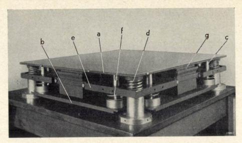
Fig. 7. Practical construction of a vibration-free mounting. The dimensions of this apparatus are  $60 \times 60 \times 15$  cm; its weight is 110 kg. The two plates a and b together form the main mass. They are connected with twelve rods c. This main mass rests upon four helical springs d. The auxiliary mass e is coupled to the main mass with eight springs f. The cup g is one of the four damping elements.
