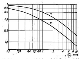
Fig. 8. The quantities  $F(\sigma/\mu) = (\sigma/\mu)^{\sigma/(\mu-\sigma)}$  and  $G(\sigma/\mu) = (^1/_2 + \sigma/_2\mu)^{\sigma/(\mu-\sigma)}$  as functions of  $\sigma/\mu$ , where  $\sigma$  represents the attenuation, are used for determining the optimum thickness of viewing screens and of front screens respectively.
