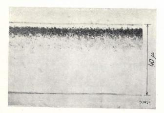
Fig. 7. Microtome cross section of a sensitized cellophane film 40 microns thick after exposure and developing. The particles of silver from which the picture is built up lie in a thin layer a few microns below the surface.
