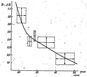
Fig. 4. Average contrast sensitivity as a function of age, measured at a level of brightness of 0.3 candle/m<sup>2</sup> in the presence of a source of glare. The glare causes a much greater decrease in sensitivity to contrast in the older age groups.
