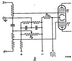
Fig. 12. The input circuit of each of the channels in the electronic switch GM 4580: a) for asymmetrical input voltage, b) for symmetrical input voltage, 0-1 input terminals for max. 50 V, 0-2 input terminals for max. 500 V, 3-4 input terminals for max. 2  $\times$  500 V.  $R_p$  is a potentiometer by means of which the oscillograms can be moved up and down.
