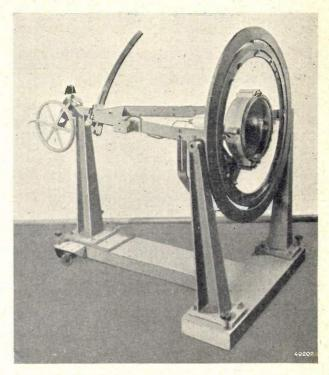
Fig. 14. The Philips measuring apparatus, with a "Philiflood" floodlight mounted in it.
