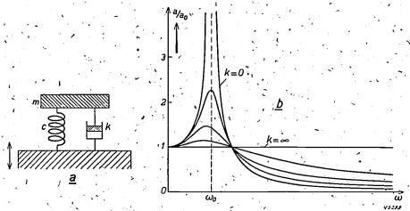
Fig. 2. Diagram (a) and frequency characteristic (b) of a vibration-free system with "relative" damping. With increasing damping (k) the resonance peak is gradually lowered and at the same time the free vibrations die out more quickly, but at high frequencies the amplitudes of the forced vibrations become larger. The amplitude ratio is given by the expression 2):
