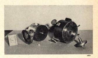
Fig. 6. Parts of a modern electron microscope. On the left a sample holder with air lock. The substance is placed on the point at the middle of the front surface of the holder. On the right an objective, and lying in front of it the holder for the objective diaphragm.
