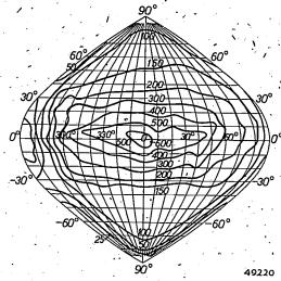
Fig. 10. The iso-candle diagram of a "Cornalux" lamp in sinusoidal projection. The luminous intensity is given in candles, whilst the total luminous flux of this light source amounts to 1320 lumens. From the diagram it may be read that this lamp, which is used for ceiling lighting, emits its light in a rather narrow beam.
