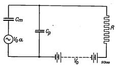
Fig. 2. The electrical circuiting of a condenser microphone in the form in which it might be regarded according to Thévenin's theorem.  $V_0$  is the voltage of the current source, R the resistor,  $C_m$  the capacity of the condenser-microphone in the state of rest,  $C_p$  the parallel capacity, and  $\alpha$  the factor determining the change in the distance between the diaphragm and the rear electrode.
