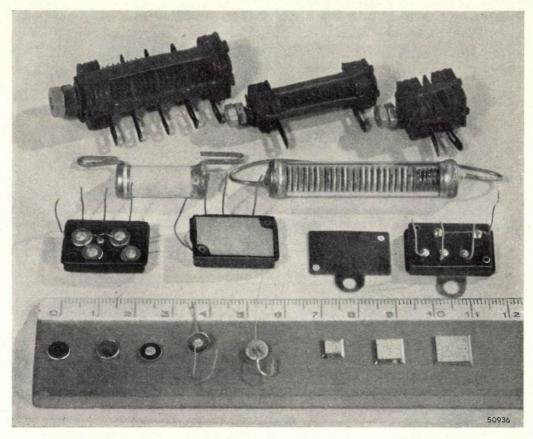
Fig. 10. Kinds of selenium rectifiers, some mounted and some not. From left to right: (front row) five cells of type I in different stages of construction (without cathode layer, with cathode layer, with lacquer and alloy, with inlet leads) and three square cells of type III;
