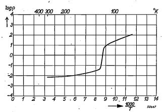
Fig. 3. Logarithm of the specific resistivity  $\sigma$  (in  $\Omega$  cm) as function of 1/T, where T is the absolute temperature, for Fe<sub>3</sub>O<sub>4</sub>.
