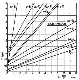
Fig. 5. Logarithm of the specific resistivity  $\sigma$  (in  $\Omega$  cm) as function of 1/T (T absolute temperature) for the mixed crystal Fe<sub>3</sub>O<sub>4</sub>-MgCr<sub>2</sub>O<sub>4</sub> for different percentages of MgCr<sub>2</sub>O<sub>4</sub>.
