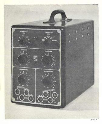
Fig. 5. The new electronic switch type GM 4580. From top to bottom: two knobs for regulating the commutating frequency, two knobs for vertical displacement of the image (left-hand one for shifting the whole image, right-hand one for shifting the two oscillograms in opposite directions), two knobs for regulating the sensitivity of the channels, terminal sockets for the symmetrical and the asymmetrical inputs.
