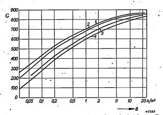
Fig. 5. The dependence of visual acuity G on the brightness B for different kinds of light, viz I for mercury light, 2 for sodium light, 3 for neon light, 4 for incandescent lamp light. The value of the visual acuity G is expressed here as the distance in cm at which circles and squares 1 cm in diameter can just be distinguished. The value G=690 thus corresponds to the capability of just seeing a detail within an angle of vision of about 1 minute.
