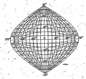
Fig. 8. For comparison some meridians and small circles of fig. 7 are shown as dotted lines on the sinusoidal projection of the grid belonging to the measuring apparatus of fig. 6.
