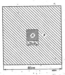
Fig. 2. The chromatic adaptation of the eye is very well demonstrated by illuminating a transparent window A with a light of a certain colour and the surrounding field B first with artificial daylight, for instance, and then with incandescent lamplight. Shortly after changing over from daylight to lamplight the eye directed upon A sees a change of colour in the window.
