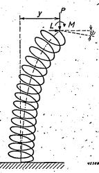
Fig. 4. When a transversally directed force L and a couple M act on the free end of a helical spring whose other end is clamped and which is compressed axially by a weight P, a lateral deflection  $\gamma$  and a rotation  $\psi$  occur at that free end.
