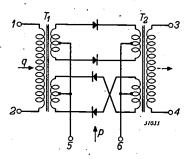
Fig. 14. Modulator in double push-pull circuit. Voltage with the audio frequencies q is applied to the terminals 1 and 2, whilst voltage with the carrier frequency p is applied to the terminals 5 and 6. The modulated voltage is taken off at terminals 3 and 4.
