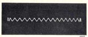
Fig. 9. a) Oscillogram of the voltage between starter and mercury cathode with a concave meniscus. There is no time lag here, although the voltage applied is very low, viz. 1.2 kV. (N.B. The time base is different from that in fig. 8 a-d!)
