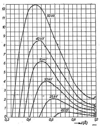
Fig. 5. Energy distribution in the continuous X-ray spectrum as a function of the wavelength  $\lambda$  for various voltages between 20 and 50 kV. With increasing tube voltage the peak of the graph is shifted to the left and the value of  $\lambda_{min}$ , the shortest wavelength in the radiation, becomes smaller. The intensity is given on the vertical axis on an arbitrary scale.
