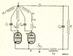
Fig. 15. Two in phase successive branches (m and l) of a rectifier with m phases provided with capacitors  $C_1 \ldots C_m$ . These capacitors reduce the ignition peaks.
