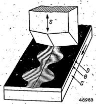
Fig. 6. Principle of the Philips-Miller system of sound recording. The "Philimil" band consists of the celluloid support C with a gelatine coating C and a very thin opaque covering layer D. The cutter s vibrating perpendicularly to the band moving in the direction of the arrow cuts out a transparent sound track.
