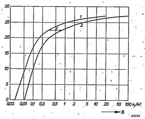
Fig. 8. The dependence of reading velocity on the brightness. As a measure of reading velocity the number of letters have been plotted which can be read per second under certain definite conditions:
