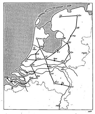
Fig. 1. The Netherlands telephone network is divided into 20 districts. The 20 district exchanges are interconnected by inter-district networks (indicated by open circles). This map shows the carrier inter-district links as used about 1940/41. The dots represent repeater stations.
