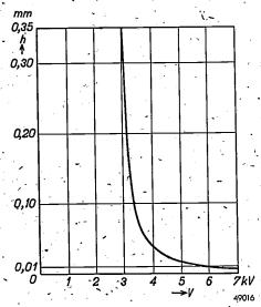
Fig. 5. Measured height h at which sparking takes place on the mercury cathode (in the case of a given igniter) as a function of the voltage V applied between the igniter (+) and the mercury cathode (-).
