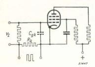
Fig. 10. The commutating voltage is conducted to the resistor  $R_k$  in the control grid circuit; the screen grid is fed in the normal manner with a direct voltage.  $C_{gk} = \text{capacitance}$  between control grid and cathode.
