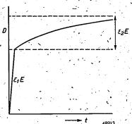
Fig. 1. The variation of the displacement D with the time t, when at time t=0 an electric field E is suddenly switched on and causes the displacement  $\varepsilon_1 E$ . The contribution caused by the adjustment of the dipoles increases gradually from zero to  $\varepsilon_2 E$ .
