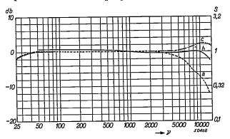
Fig. 4. Three characteristics showing that the damping can be regulated by adjusting the distance between the diaphragm and the rear electrode:
