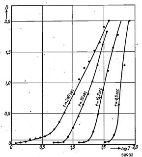
Fig. 5. From the density plane drawn in fig. 4 it is possible to find for any exposure time t the density curve D = f(I) of the picture obtained with that exposure time, by taking a cross section of the plane perpendicular to the t-axis at the level of that time. Such cross sections are represented here for various exposure times. It is seen that curves are obtained with different slopes (different gammas).
