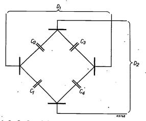
Fig. 6.  $C_1$ ,  $C_2$ ,  $C_3$  and  $C_4$  are the stray capacities between the deflecting plates (and their leads) belonging to different pairs. Through these capacities the pairs of plates  $D_1$  and  $D_2$  are apt to exercise an adverse electrical effect upon each other.
