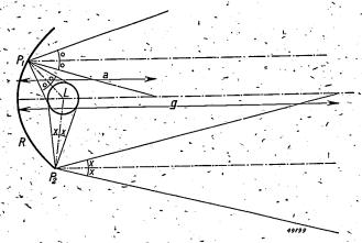
Fig. 4. A spherical light source L with its centre in the focus of the reflecting rotational paraboloid R. None of the light in the beam reflected at  $P_1$  will reach the axis within a distance afrom the reflector. For a point  $P_2$  on the edge of the reflector reaches its maximum value g, called the photometrical boundary distance.
