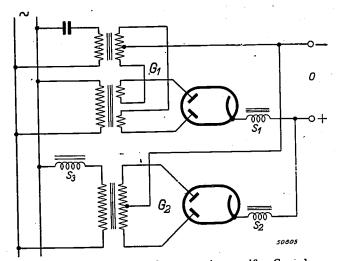
Fig. 9. Parallel circuiting of a preserving rectifier  $G_1$  and an ordinary rectifier  $G_2$ . In the special case where we applied this arrangement it was desirable to use rectifying valves instead of selenium valves.  $S_1$  and  $S_2$  are chokes.  $S_3$  is a variable choke by means of which the flat part of the resulting characteristic (see  $G_1 + G_2$  in fig. 10) can be shifted to the desired current intensity range.
