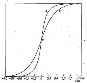
Fig. 2. The luminous intensity curve in the image of the edge of a metal plate on a film obtained with the aid of a fluorescent screen; a) when using an intensifying screen of fine-grained calcium tungstate; b) with a viewing screen of coarse-grained zinc-cadmium-sulphide. Both curves are symmetrical with respect to point M, corresponding to point B in fig. 1.
