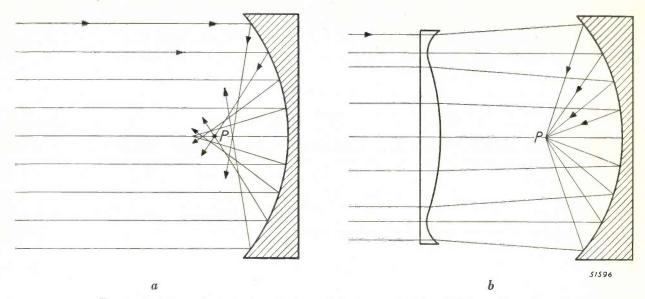
Fig. 4. a) With a spherical mirror the rays of the beams at different distances from the optical axis converge at different points.
