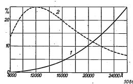
Fig. 4. Transmission of infra-red rays when drying lamps are used for lacquers. Curve I gives an idea of the transmission of a certain kind of lacquer for infra-red energy of different wavelengths. For comparison curve 2 gives the spectral energy distribution of the Philips drying lamp.
