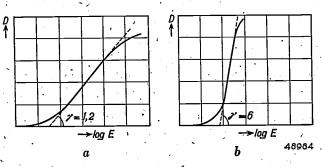
Fig. 3. H & D curve for a photographic negative or positive represented diagrammatically. D= density, E= exposure (= exposure intensity  $\times$  exposure time),  $\gamma=$  slope of the rectilinear portion of the curve. The gamma depends upon the kind of film and the method of developing. a) The case of a low gamma; b) the case of a high gamma.
