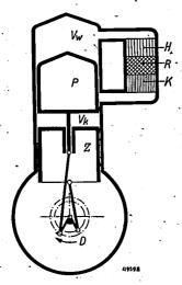
Fig. 5. Diagram of an air engine with transfer piston where only one cylinder is used. For the meaning of the letters see figs. 4 and 1.
