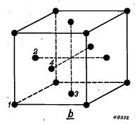
Figs. 1 a) and b): Two possible choices of the elementary cell of the oxygen ion lattice in spinels. The large black dots indicate oxygen ions. b) is formed from a) by shifting all the lattice points parallel to the body diagonal on which oxygen ion 1 is sivated.
