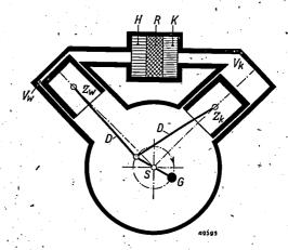
Fig. 3. Diagram of an air engine according to the so-called V-construction. The letters have the same meaning as in fig. 1. G = counterweight. Advantages: simpler drive, closed crankcase (possibly with elevated pressure), balanced inertia forces of the pistons.
