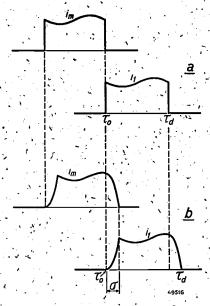
Fig. 10. Commutation of the current from branch m to branch l.
