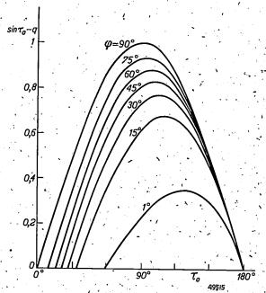
Fig. 5. The factor ( $\sin \tau_0 - q$ ) by which the voltage impulses upon ignition are proportional, as function of the ignition angle  $\tau_0$ , with  $\varphi$  as parameter. Large values occur at  $\varphi \approx 90^\circ$  (strongly inductive circuit) and  $\tau_0 \approx 90^\circ$  (ignition at the top of the alternating voltage).
