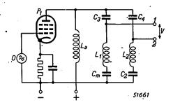
Fig. 5. System for feeding the two bridge branches  $(L_1\text{-}C_m \text{ and } L_2\text{-}C_2)$  of fig. 4. 0 is an oscillator with the carrier-wave frequency,  $P_1$  an amplifying valve (pentode),  $C_3$  and  $C_4$  are condensers in series with the two branches,  $L_a$  is a coil in resistance with  $C_3$  +  $C_4$ , 1 and 2 are the terminals across which the modulated voltage arises.
