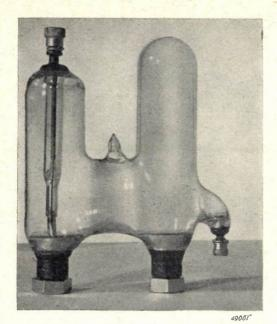
Fig. 13. Relay valve with mercury cathode (left) and dielectric igniter. The anode and the auxiliary anode (right) also consist of mercury in order to avoid contamination of the igniter. The valve, which is about 18 cm in height, can transmit current impulses of 2000 amp. In view of the permissible temperature, the average current is limited to about 1.5 amp. with natural cooling of the valve, and to about 3.5 amp. when a fan is used.
