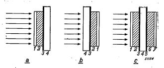
Fig. 2. Diagram showing how intensifying screens are used. a) front screen, b) back screen, c) front and back screens. I and 7 cardboard base, 2 and 6 fluorescent layer, 3 and 5 sensitized layer, 4 celluloid.
