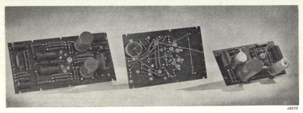
Fig. 12. Units mounted on insulating panels: on the left one of the push-pull amplifiers (rear view), in the middle the other amplifier (rear view), on the right the generator for the time-base voltage. (The two amplifier panels are not equal in size because on one of them some other parts are mounted which belong to the supply part.)
