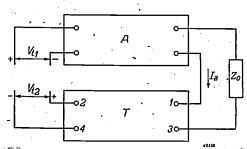
Fig. 1. If for a certain frequency the transfer impedance  $Z = V_{t_2}/I_a$  of the feedback network T assumes the value -1/S (S = slope of the amplifier A,  $= I_a/V_{t_1}$ ) then the voltage supplied by T is just identical with the voltage required at the input of the amplifier to produce  $V_{t_2}$ . When the output of T is connected to the input of A the amplifier starts oscillating in that frequency.
