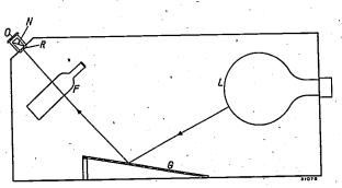
Fig. 5. A strain-viewer for determining and measuring stresses in glass articles. With the aid of a glass plate G the light from the lamp L is polarized and passes through the glass bottle F being tested, a red plate R and a nicol N, reaching the observer's eye through an eye-piexe O. The stresses present in the bottle can be determined by comparing the colour of the field before and after introducing the bottle.
