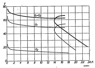
Fig. 8. Characteristics of the two rectifiers of fig. 7, each taken separately:  $G_1$ ,  $G_2$ ; the resulting characteristic of the series connection of the two rectifiers is  $G_1 + G_2$ .
