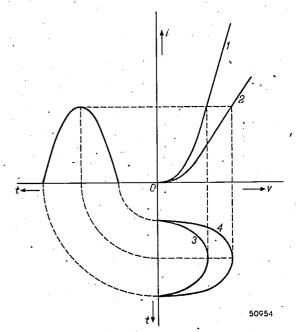
Fig. 12. (1) and (2) are characteristics of the current i in the transmitting direction as functions of the voltage v of two similar cells whose effective surfaces are as 2:1. The voltage loss in the cells when the same current passes through (current i represented on the left as function of the time t) is given by the curves (3) and (4). The amplitude of (4) is less than twice that of (3).
