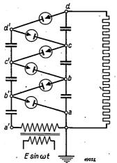
Fig. 2. The circuit of a cascade generator having six valves, which furnishes the no-load voltage 6E at d when the amplitude of the a.c. voltage given by the transformer is E. In the circuits ab', b'b, etc. are the six valves for 150 kV negative anode voltage.
