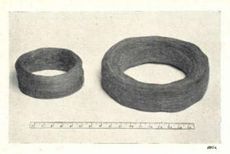
Fig. 4. Two regenerators for engines of  $3^{1}/_{2}$  and 10 h.p. respectively. In the Philips air engines the air flows from the hot to the cold space through an annular shaped channel in which the regenerator is placed. (The scale is in centimeters.)
