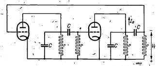
Fig. 8. Example of a system (see footnote 2) without oscillating circuit, which can still oscillate (so-called RC generator).
