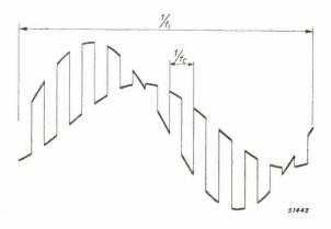
Fig. 2. Picture of two sinusoidal input voltages as it appears on the oscillograph with the circuiting according to fig. 1 when the commutating frequency  $f_c$  is higher than the frequency  $f_i$  of the input voltages. In reality  $f_c$  is much higher than is represented here.
