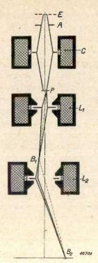
Fig. 7. The path of the rays of a magnetic electron microscope. E is the source of electrons, A the anode, C the condenser,  $L_1$  the objective,  $L_2$  the projector, P the object,  $B_1$  the intermediate image,  $B_2$  the final image.
