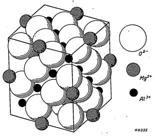
Fig. 4. Elementary cell of spinel proper, MgAlO<sub>24</sub>. It may be seen that the oxygen ions are much larger than the metal ions.
