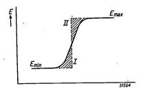
Fig. 6. The luminous intensity E in the image of an edge is distributed, owing to screen blurring, according to an S-shaped curve. Ne met, Cox and Walker take the sum A of the areas I and II for defining the screen blurring, putting  $u_s = 4A_i (E_{\max} - E_{\min})$ , where  $E_{\max}$  and  $E_{\min}$  are respectively the maximum and the minimum luminous intensities in an edge image on a film.
