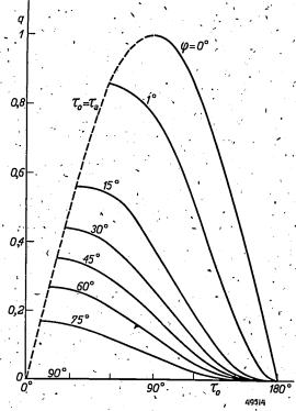
Fig. 4. The relation q (approx. equal to the direct voltage  $V_0$ ' divided by the top value  $V_{\max}$  of the alternating voltage) as a function of  $\tau_0$ , with  $\varphi$  as parameter. The dotted line again corresponds to the earliest possible ignition  $(\tau_0 = \tau_a)$ .
