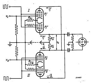
Fig 8. Both channels of fig. 1 in push-pull as indicated in fig. 7 for channel I. The pentodes  $P_{I}$  and  $P_{I}$ ", respectively  $P_{II}$  and  $P_{II}$ ", can be replaced by a double pentode (type EFF 52).
