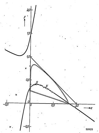
Fig. 4. Experimentally determined points of intersection  $(\times)$  of corresponding rays in the two pencils of rays centered on G and K. The locus of the points of intersection may by approximation be represented by a hyperbola. With the hyperbola most closely matching the emperical points (drawn in the figure) the standard error of the "predicted" hue number N is only 0.42.
