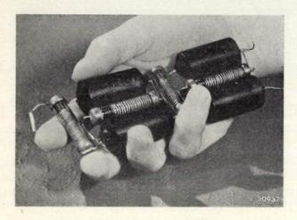
Fig. 15. Cascade connection consisting of four tubes, each containing about 25 selenium cells in series, and four capacitors. With this device the direct voltage of 1200 volt is obtained from 220 V alternating voltage.
