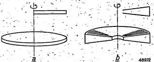
Fig. 5. The formation of a round flat cavity resonator by the rotation of a Lecher system short-circuited at one end: a) plane cavity resonator, b) resonator of a more general form.
