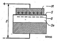
Fig. 4. The voltage E in the circuit of fig. 3 causes charges on either side of the blocking layer S, positive in the metal at M and negative in the semi-conducting selenium Se. This gives rise to an area G in the latter layer where all open places are occupied by electrons and which consequently no longer has any conductivity, This area G becomes thicker the higher the voltage E, which accounts for the drop then found in the capacity.
