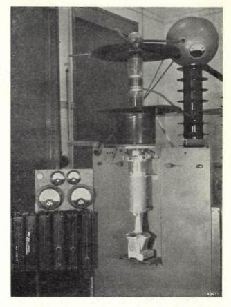
Fig. 4. The microscope proper with the acceleration tube. The protecting plate has been removed to show clearly the acceleration tube. On the right is a column containing the resistances for the potentiometer from which the current for the tube is tapped. On top of this column, in a metal sphere at a potential of —400 kV with respect to earth, is a 6-volt accumulator for the heating of the filament.
