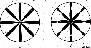
Fig. 2. Representation of the fundamental oscillation (a) and of a higher characteristic oscillation (b) of a round plane cavity resonator. A few current lines have been drawn whose width is proportional to the current density. Due to the rotational symmetry all the "lines" are congruent.
