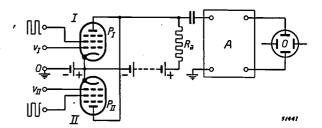
Fig. 1. Circuiting diagram of an electronic switch. I and II are channels functioning alternately for carrying the input voltages  $v_I$  and  $v_{II}$  to the amplifier A and the oscillograph tube O.  $P_I$  and  $P_{II}$  are pentodes,  $R_a$  is a common anode resistance.
