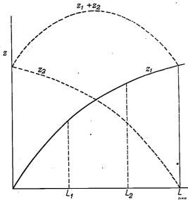
Fig. 9. Graphical representation of the blackening z as function of the light energy L according to formula (17). It is seen that  $z(L_1) + z(L_2) > z(L)$  for  $L_1 + L_2 = L$ . The left-hand member of this inequality reaches its maximum for  $L_1 = L_2 = L/2$ .
