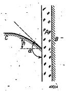
Fig. 2. Shape of the mercury meniscus at the igniter. The letters A, B and C have the same meaning as in fig. 1b. a is the so-called boundary angle, which varies for different substances and for the combination mercury-quartz amounts to about 135°. The position of a point on the convex mercury surface is determined by the height h above the boundary line between the mercury and the wall of the igniter.
