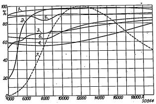
Fig. 5. The reflection coefficient, expressed as a percentage of the incident energy, of some metals that could be used as mirror of a drying lamp, I is silver, 2 gold, 3 nickel, 4 chromium, 5 evaporated aluminium and 6 polished aluminium. For comparison curve 7 gives the spectral energy distribution of the radiator.
