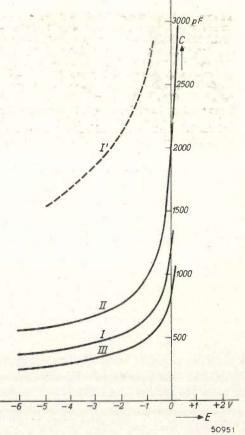
Fig. 8. The capacity C measured with the circuiting scheme of fig. 3 plotted as a function of the applied direct voltage E, for the rectifiers I, II and III. The curve I has been derived by multiplying the ordinates of I by 4.
