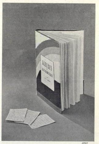
Fig. 11. Three small sheets of metal-diazonium paper on which the complete contents of a book of 330 pages have been reduced. Each page of the book is reduced on the paper to a size of  $5 \times 7$  mm. The reproduced book is quite legible with a simple reading apparatus.
