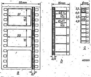
Fig. 4. The three sizes of film commonly used: 35, 16 and 8 mm wide. For each film the width and height of the photographed picture frames are given, the slightly smaller width and height of the film gate in the projector (thus the dimensions of the picture to be projected) and the width of the sound track.
