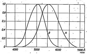
Fig. 9. Eye sensitivity (in relative units) as a function of the wavelength (in  $\dot{A}$ ) for cone vision (A) and for rod vision (B).
