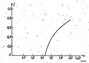
Fig. 6. The relation between the compression  $\xi$  and the ratio of slenderness  $l_0/D$  which follows from the condition that the spring must have the same axial and lateral rigidity.
