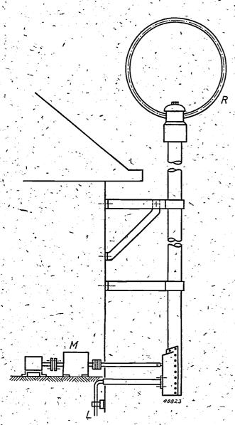
Fig. 9. Setting up the frame aerial on a huilding. R = frame aerial (one winding of copper tubing; diameter at least 1 m). M = motor turning the frame. L = transmission line connecting to the receiver.
