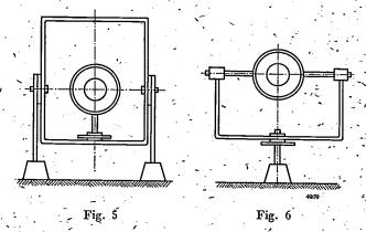
Fig. 5. A measuring apparatus where the projector turns about a fixed horizontal axis and also about an axis which in the position of rest is vertical and upon rotation follows the movement of the horizontal axis. Fig. 6. A measuring apparatus where the light source turns about a fixed vertical axis and also about a horizontal axis following the movement of the vertical axis.
