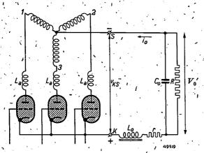
Fig. 8. Circuiting of a rectifier fed from a three-phase system of alternating voltages.  $L_a = \text{leakage}$  inductance per branch.
