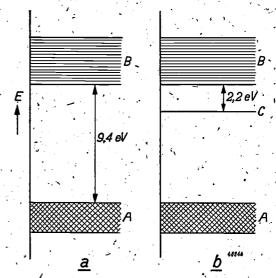
Fig. 4. Simplified diagram of energy bands:
