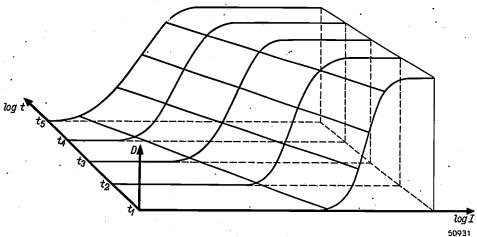
Fig. 4. The gamma of the metal-diazonium system also depends, i.a., upon the intensity of exposure I. Therefore the density D is not fully determined by the product I is the photographic behaviour of the system has to be described by a solid density plane D = f(I, t). This plane is drawn here for given concentrations, moisture content, developing, etc. in perspective. Log I and  $\log \iota$  are plotted as independent variables.
