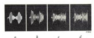
Fig. 12. Oscillograms recorded with the apparatus according to fig. 8. Duration of the sound impulses: (a) 0.12 sec., (b) 0.07 sec., (c) 0.035 sec., (d) 0.02 sec. Pitch 1072 c/s. The width of the oscillogram corresponds to 0.54 sec. Since it was not necessary in this case to adjust as accurately as possible the constant amplitude, this was only done approximately.
