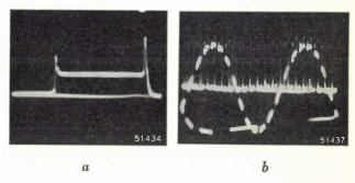
Fig. 3. a) Oscillogram of the output voltage of the amplifier of the oscillograph GM 3152 with the old electronic switch GM 4196 connected in front of it, the two input voltages of the latter being zero. The voltage obtained (frequency about 8000 c/s) deviates rather considerably from the rectangular shape, this being due, inter alia, to a peak arising at each commutation.
