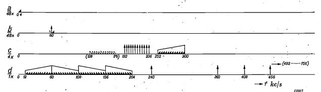
Fig. 5. Complete modulation diagram of the 48-channel system. (a) Audio-frequency channel. (b) Terminal modulation and basic channel. (c) Channel modulation and basic group. (d) Group modulation and 48 channel super-group.
