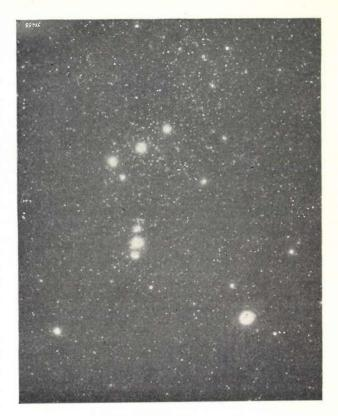
Fig. 7. Part of the Orion constellation as photographed in the Philips laboratory at Eindhoven when using a Schmidt mirror system (focal distance 8 cm) with a correction plate of gelatin. This photo demonstrates the large useful field of vision. Although its diameter is about 20° the image is sharp and free of aberrations right up to the edges of the photo.
