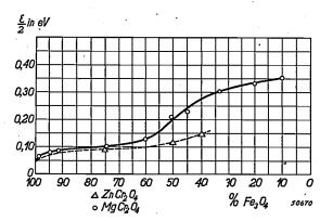
Fig. 6. The activation energy  $\varepsilon$  (in eV) as function of the percentage of Fe<sub>3</sub>O<sub>4</sub> for mixed crystals of Fe<sub>3</sub>O<sub>4</sub>-ZnCr<sub>2</sub>O<sub>4</sub> (broken line) and Fe<sub>3</sub>O<sub>4</sub>-MgCr<sub>2</sub>O<sub>4</sub> (fully-drawn line).
