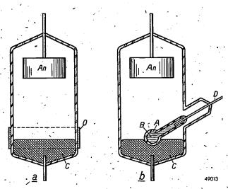
Fig. 1. a) The ignition band (0) of Cooper Hewitt is a metal band laid around the outside of the glass discharge vessel at the height of the meniscus of the mercury cathode C. A voltage impulse of about 10 kV applied to 0 and positive with respect to C causes a cathodc spot on the mercury near the glass wall, after which a discharge to the anode An develops which further maintains the discharge.
