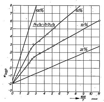
Fig. 4. Logarithm of the specific resistivity  $\sigma$  (in  $\Omega$  cm) as function of 1/T (T absolute temperature) for the mixed crystal Fe<sub>3</sub>O<sub>4</sub>-ZnCr<sub>2</sub>O<sub>4</sub> for different percentages of ZnCr<sub>2</sub>O<sub>4</sub>.
