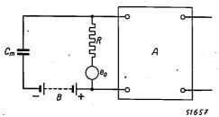
Fig. 1. Conventional circuit of a condenser-microphone  $(C_m)$ . B is a source of direct voltage, R a resistor of high impedance, A an amplifier;  $e_o$  represents the noise voltage coming from R.
