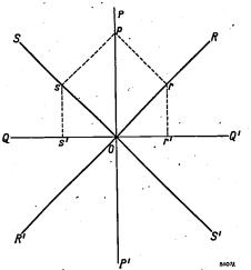
Fig. 4. The wave directions of the crystal (RR' and SS') make an angle with those of the niclos (PP' and QQ'). Of a wave Op that has passed through the polarizer, the analyzer allows the components Or' and Os' to pass through. These components will interfere.
