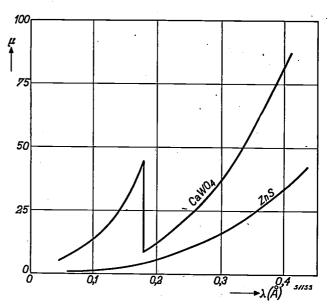
Fig. 4. Graphical representation of the absorption coefficient  $\mu$  (in cm<sup>-1</sup>) as function of the wavelength  $\lambda$  (in Ångström) for CaWO<sub>4</sub> and ZnS.
