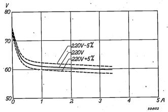
Fig. 6. Characteristics as in fig. 5 for three different mains voltages (nominal 220 V). Only the flat branch is drawn. It will be noted that the voltage rises with falling mains voltage and vice versa. The variations are small: about 3% for 10% mains voltage variation.
