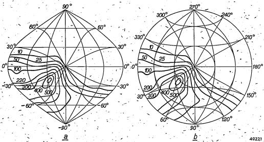
Fig. 12. The iso-candle diagram of a light source for road lighting (fitting Philips ZE 30) in a) sinusoidal projection and b) azimuthal projection according to Lambert. The other hemisphere is symmetrical with the one represented here. The luminous intensity is given in candles for a light source with total luminous flux of 1000 lumens.
