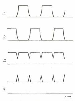
Fig. 6. Trend of the two anode currents (a and b), the current (c) through the resistance  $R_a$  and the anode voltage (d) in the circuit according to fig. 1, with equal and constant values of  $v_I$  and  $v_{II}$ .
