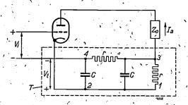
Fig. 2. Example (see footnote  $^2$ ) of an amplifier with feedback system T consisting of two resistances r and two capacitors G. The numbering I-4 of the terminals of T corresponds to that of fig. 1.
