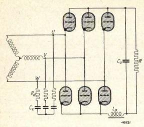
Fig. 12. Circuit according to Grätz, the voltage on which between the points U and V is represented in the oscillograms of figs. 13 and 16. The functions of the capacitors  $C_x$  and the damping resistance  $R_d$  will be discussed farther on.
