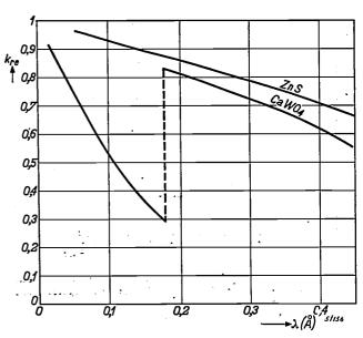
Fig. 6. The yield  $k_{re}$  from the conversion of X-rays into electron energy as function of the wavelength  $\lambda$  for CaWO<sub>4</sub> and ZnS.
