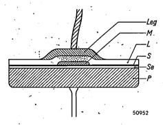
Fig. 9. Cross section of a cell of type I. P= carrier plate, Se= selenium layer, S= genetic blocking layer, M= cathode obtained by vaporization, L= lacquer, Leg= alloy for soldering the inlet lead. The lacquer allows enough of the alloy to pass through to ensure a good electric contact; the obnoxious Cd-Se compound is formed on only a very small part of the effective surface.
