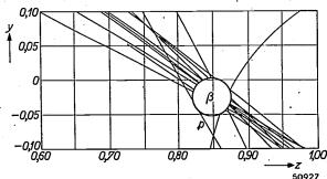
Fig. 6. Determination of the "bluepoint"  $\beta$  from the series of conic sections, derived from the comparison of the light sources D and I-5 with G and with K (observer B).
