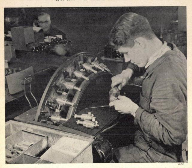
The final processes in the manufacture of cycle dynamos are the running in, the adjustment of the driving wheel (reducing the axial play to the minimum) and the mechanical and electrical testing.
