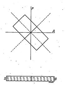
Fig. 8. The manner in which a test plate of glass G fused onto a standard glass S is placed in the polarizing microscope. P and A are the respective directions of the waves allowed to pass through the polarizer and the analyzer.
