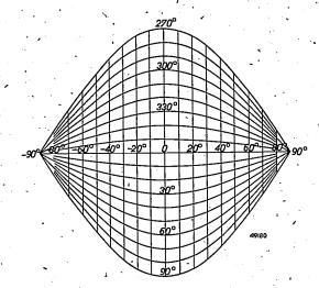
Fig. 7. The sinusoidal projection of the grid belonging to the measuring apparatus of fig. 5.
