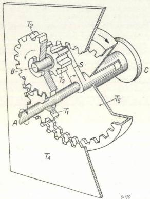
Fig. 2. Schematic drawing of the new epicyclic gearing in perspective. For the meaning of the letters see the text and explanation of fig. 1.
