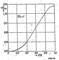
Fig. 16. The lowest but one characteristic frequency  $\omega''$  plotted vertically of the cavity resonators coupled by a hole as a function of the ratio  $\varrho/R$  (plotted horizontally), of the radius  $\varrho$  of the hole and the radius R of the cylinder. The dotted part of the curve is not well known theoretically:
