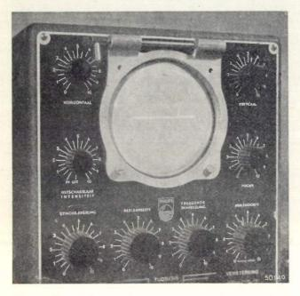
Fig. 5. The voltage impulses generated by the ticking of the watch are visible on the screen of the oscillograph in the shape of peaks, which if the watch is keeping correct time appear at the same place every time but shift when the watch is gaining or losing. The speed at which the peaks shift is a measure for the deviation from the correct time-keeping. Even a small deviation can already be measured in a few minutes.
