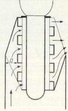
is situated inside the air inlet tube. Through the openings indicated by O around the cooling fins only half as much air now flows as in the design according to figs. 3 and 4; as a result in the case of fig. 9 these openings can now be made smaller without involving a higher air resistance, which results in smaller dimensions of the cooler housing and thus a smaller anode capacity.
