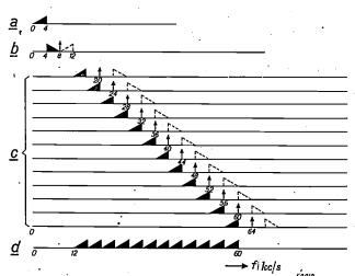
Fig. 8. Modulation diagram of a 12-channel system developed Germany. Double modulation is used but with a basic channel at 4-8 kc/s below the final group (12-60 kc/s.)
