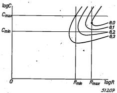
Fig. 8.  $R_{\min}$ ,  $R_{\max}$ ,  $C_{\min}$ ,  $C_{\max} =$  limits between which the value of one resistor R or of one capacitor C respectively may lie in the diagram of fig. 7; the other components have the prescribed values. With log R and log C as coordinates the lines of constant amplification are the curves indicated. It is seen that the smallest amplification (8.0) is obtained when C has a value between  $C_{\min}$  and  $C_{\max}$ .
