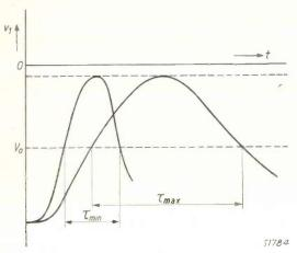
Fig. 6. Trend of the bias  $v_1$  generated in the system of fig. 5 The time during which this bias exceeds the grid voltage  $V_0$  at which the valves  $P_6$  and  $P_7$  (fig. 5) are blocked is variable between  $\tau_{\min}$  and  $\tau_{\max}$ .
