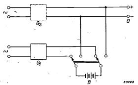
Fig. 2. Emergency supply system with only one battery and two rectifiers. While the plant connected at O is being fed from the rectifier  $G_2$  (sometimes direct supply from the mains is also possible) the battery B is being kept under a preserving charge from its own rectifier  $G_1$ . In the event of the mains failing B is switched over to the plant.
